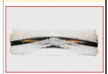
**Main Scrubbers** use a full-fill design that keeps bristles on the surface at all times. The "V" pattern that is used on most brushes directs the solution to the center of the scrubbing path as the bristles agitate the debris loose from the ground. The filament length on this brush designates it as a "scrubber" since the short bristle isn't able to "flick" or "sweep" the debris off the ground.
